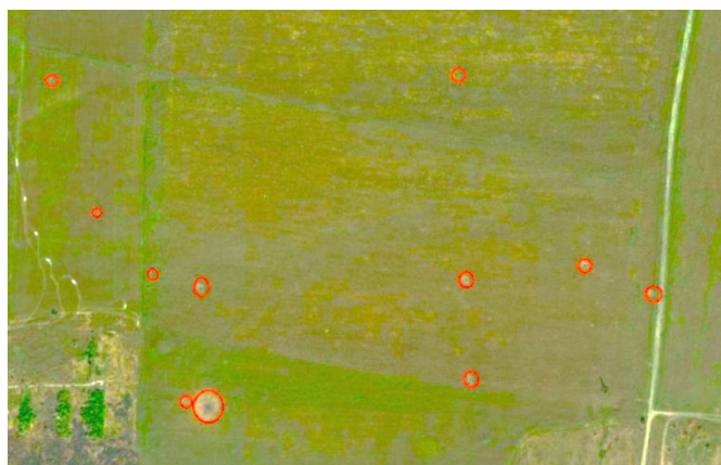
Fig. 9. Example of identifying craters on agricultural lands based on an orthophoto
