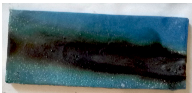
Fig. 3. The sample of the DGEBA/PEPA-CuSiF 6 after combustibility testing
