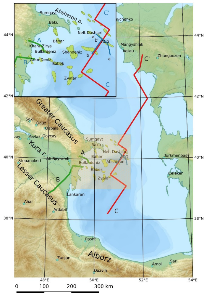
Fig. 1. General layout of SCB, modeling profiles and major oil&gas fields. Red line (C-C'): regional SW - NE profile, Figs. 4, 5; blue lines (inset, a-a', b-b'): profiles used in local migration model of ACG field, Fig.6, a, b
