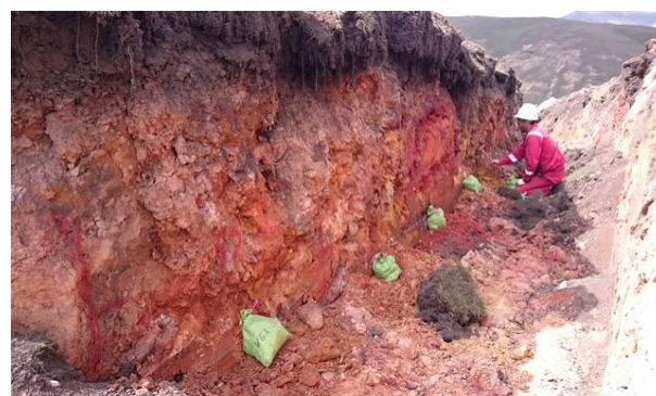
Fig. 5. Controlling of exploration surface sampling of trenches Reza gold deposit of Ugur Exploration Area
