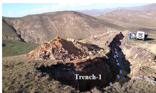
Fig. 5. Controlling of exploration surface sampling of trenches Reza gold deposit of Ugur Exploration Area
