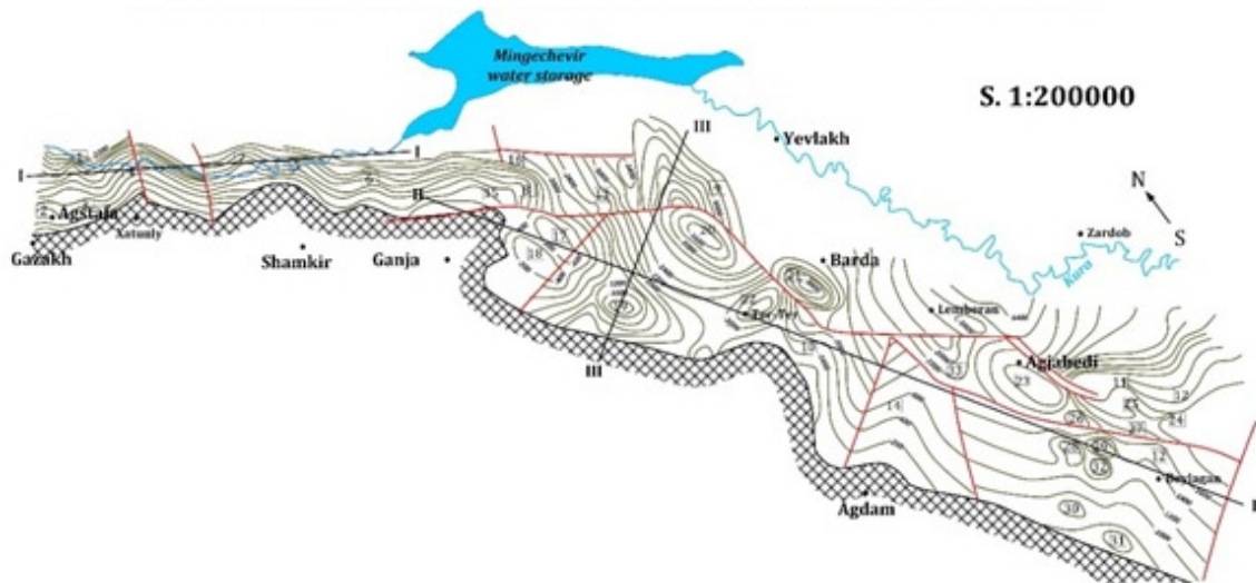
Fig. 6. Structural map by the surface of the Eocene of the Cis-Lesser Caucasian trough (composed by Pogorelova, 1991)
