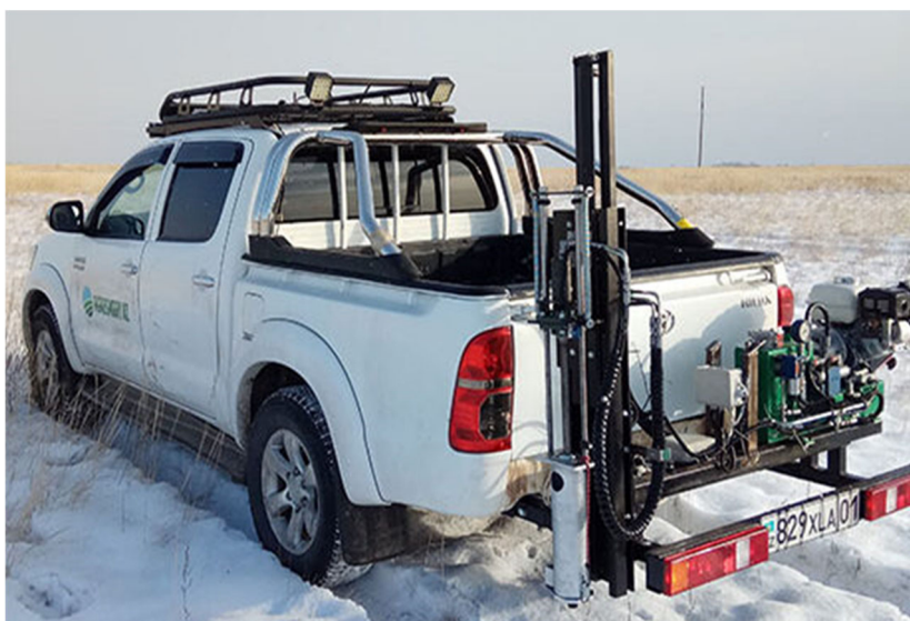
Fig. 4. Automatic Soil Sampler AgriSoilSample by the Ukrainian Company Agrilab (Soil Sampler AgriSoilSample, 2024)
