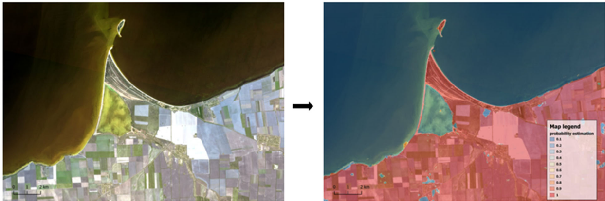
Fig. 8. The result of coastline detection using semantic segmentation, which is represented as a probability raster dated as of 01.07.2022
