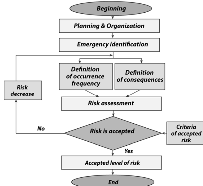
Fig. 2. Block-diagram of analysis of emergency risk occurrence
