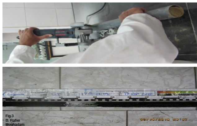
Fig. 3. Cutting of polyethylene pipes by means of milling machine (above) and sedimentary cores after cutting (below)
