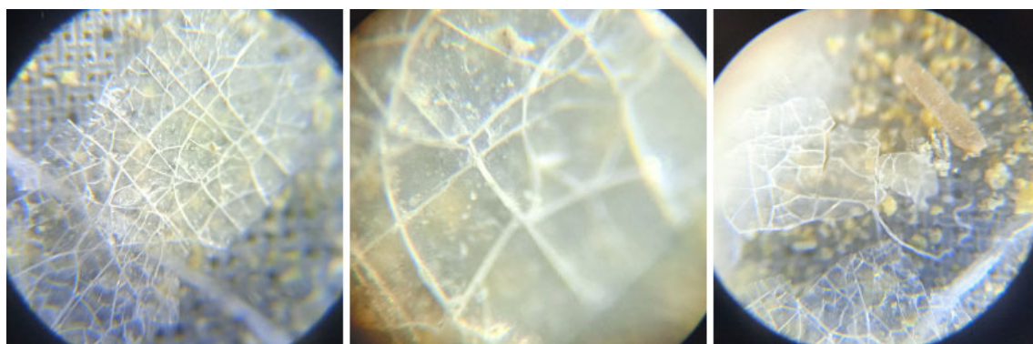
Fig. 9. A microplastic (polypropylene) fragment that resembles a strip in shape (1), its texture in the enlarged photo (2), and sample fragments (3)
