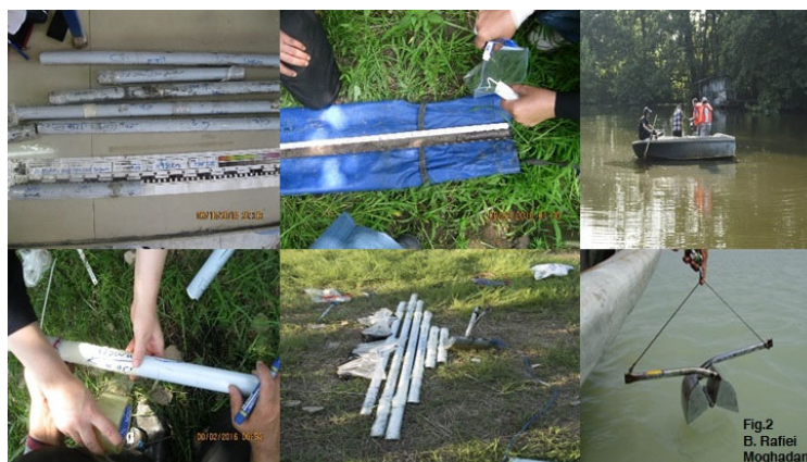
Fig. 2. Coring the wetland using polyethylene pipes, and packing and recording the cores (left), and sampling by grab (right)
