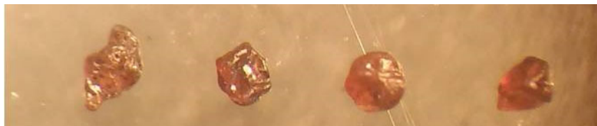
Fig. 17. Stavalite grains under a binocular microscope, 0.25–0.5 mm fraction
