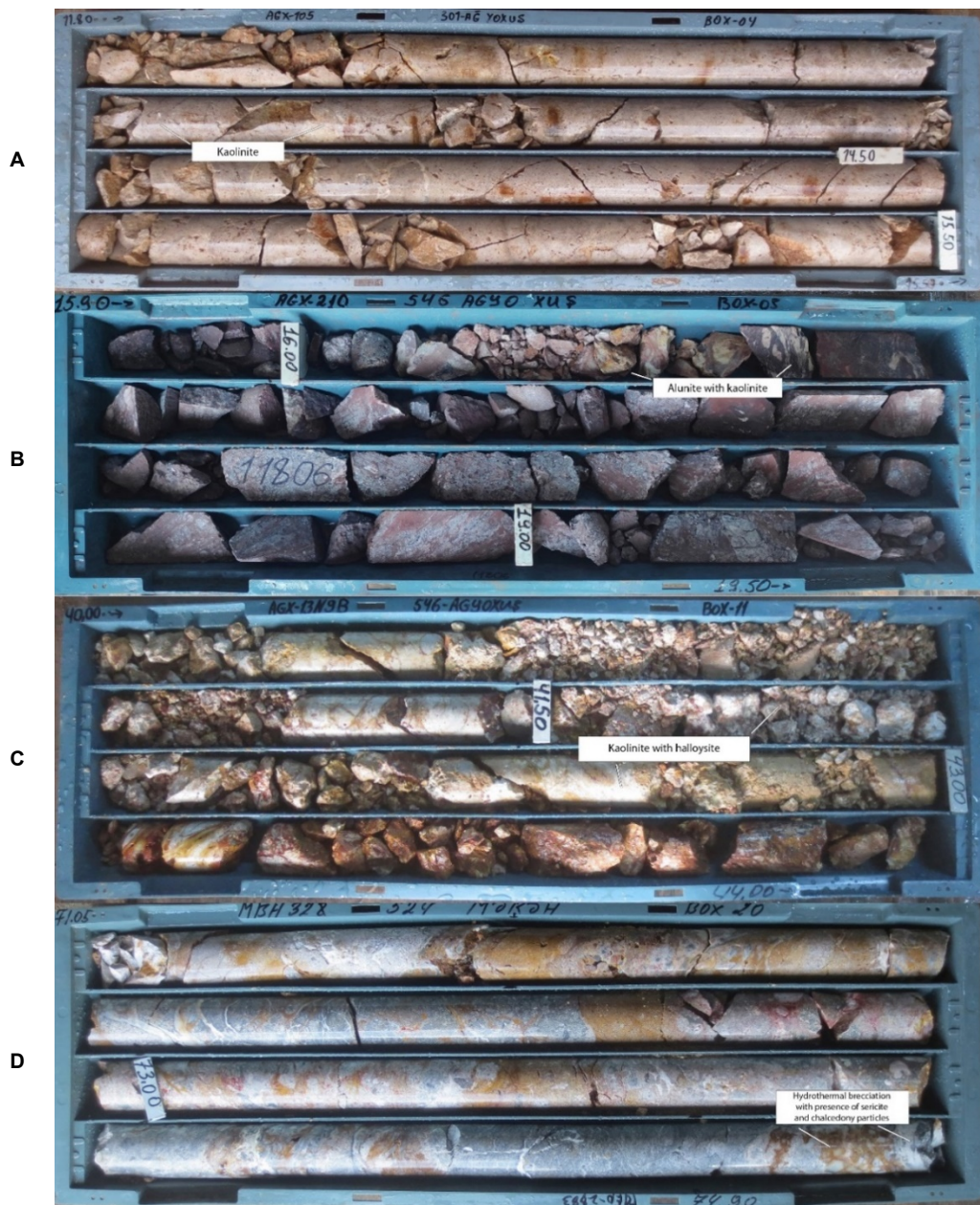
Fig. 3. (A) Representative core samples from the orebody of the Aghyokhush-1 deposit.
