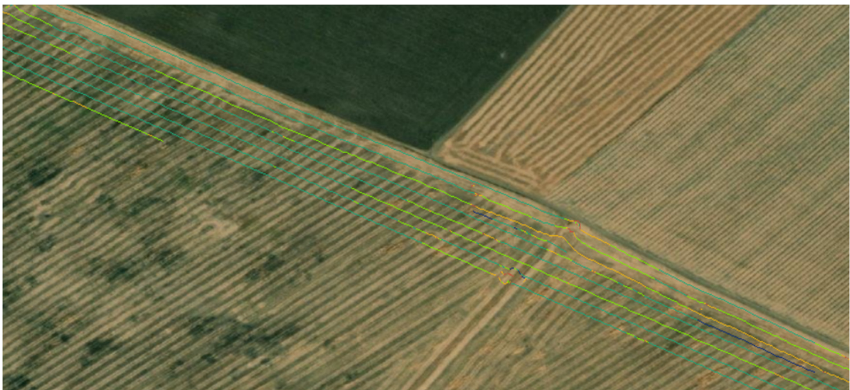
Fig. 6. Spatial distribution of segmented GNSS-based machinery movement trajectories within the study field
