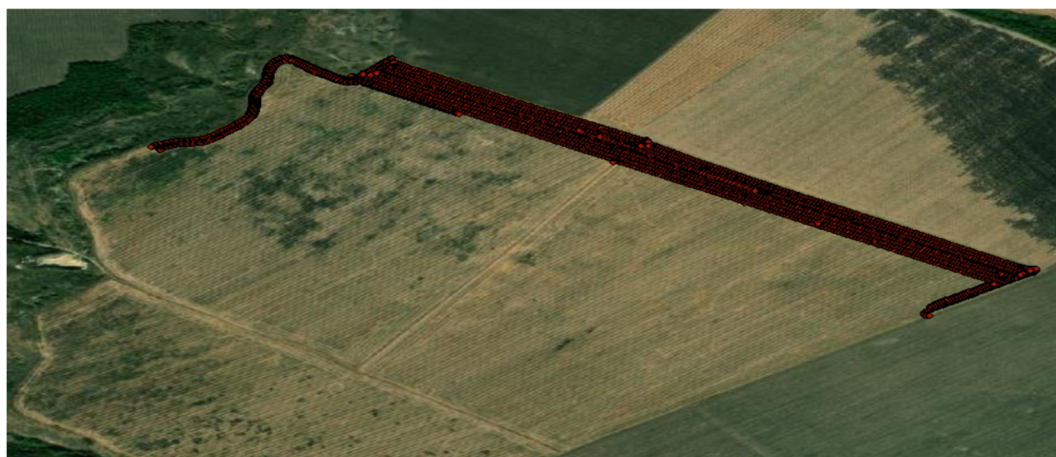
Fig. 3. Subsample of GNSS points (n=5,000) used for further calculations of machinery movement parameters (John Deere models S770 and S670)
